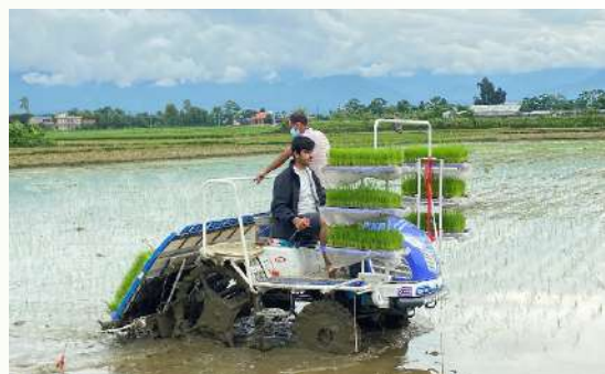
Figure: 4 wheel drive 6 row riding type rice transplanter in operation in Chitwan
